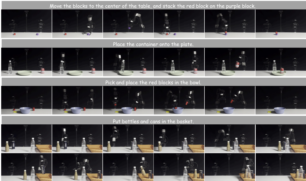
Figure 9. Qualitative results of BehaviorVLA on Real-World. From top to bottom, we illustrate four Long-horizon Tasks : Move and stack blocks on center , Place containers on plate , Pick and place blocks in bowl , and Place bottles and cans in basket . By conditioning the policy on a global prototype for structural guidance and dynamically tracking execution via phase variables, BehaviorVLA mitigates temporal drift, ensuring that local actions remain synchronized with the overall task progress.
